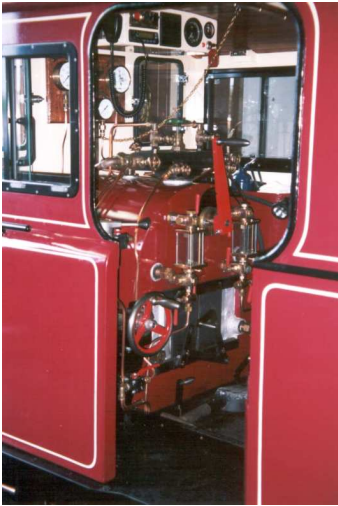
Figure 17. The new cab layout showing the ergonomic positioning of controls which was the subject of favourable comment by the Railway Inspectorate during type approval trials. The use of LED illumination of gauges makes night time operation comfortable for crews and avoids reflected glare and the hassle associated with traditional oil lamps.
