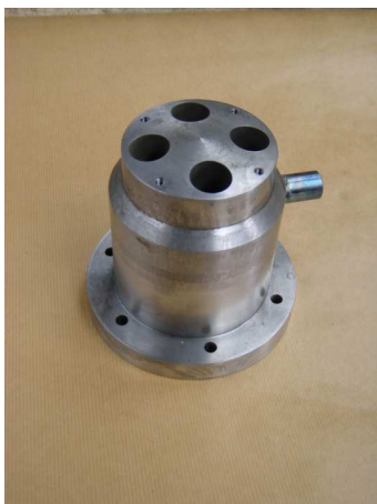
Figure 14. The four nozzle blast cap with integral blower. The blast nozzles are of the convergent divergent type to maximise the coefficient of discharge and minimise the exhaust back pressure. The nozzles are also angled outwards to ensure that the blast fills the mixing chamber of the chimney evenly.
