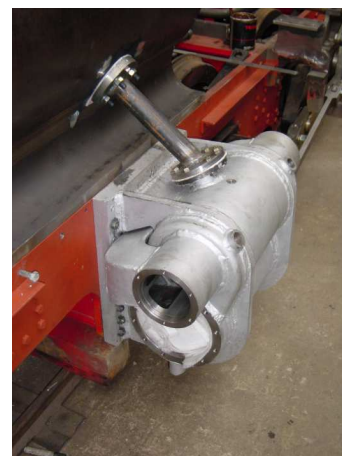
Figure 15. One of the new cylinders in place with the steam pipe connected but without the lagging or end covers. The large rectangular exhaust passageway sweeping back from the front of the valve chest can be clearly seen.
