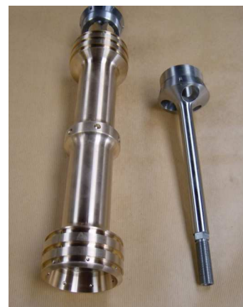
Figure 8. The hollow bronze valve heads are mounted on stainless steel valve and tail rods which are through ported to improve exhaust release and relieve loads on the valve gear. Bronze was selected for the valve heads as it provides a good wear combination with the cast iron liner. Stainless steel was selected for the rods as it had a similar coefficient of thermal expansion as the valve head and therefore would not loosen in service while also providing excellent corrosion resistance when the locomotive is laid up over the winter period preventing damage to gland packing.
