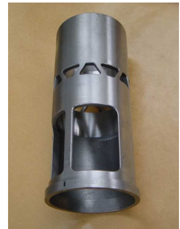
Figure 11. One of the new split cast iron valve liners showing the trapezoidal transfer ports and large exhaust ports. Two liners are required per valve chest one being inserted from each end leaving a gap between them in the centre of the steam chest for passage of live steam to the valve head. As with the cylinder liners they are sealed to the cylinder fabrication using Aflas O rings and are clamped in position by the valve chest covers.
