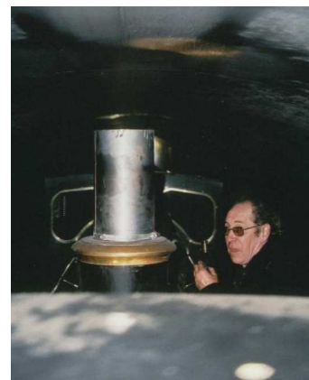
Figure 7. Bure Valley Railway CME, Dave Phillips, checking the clearances with an increased chimney height in Aylsham Tunnel using No. 7 as a testbed.
